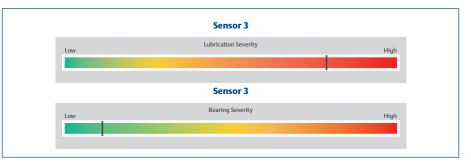
*PeakVue Plus prescriptive analytics show that this machine has insufficient lubrication, but the bearing has not been damaged yet.*
